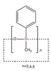
PhD3: Trimethyl-triphenyl-cyclotrisiloxane 20~30% PhD4: Tetramethyl-tetraphenyl-cyclotetrasiloxane 55~65% PhD5: Pentamethyl-pentaphenyl-cyclopentasiloxane 10~20%
